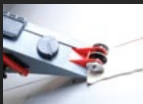
Run Wallboard Taping Tool along the joint
